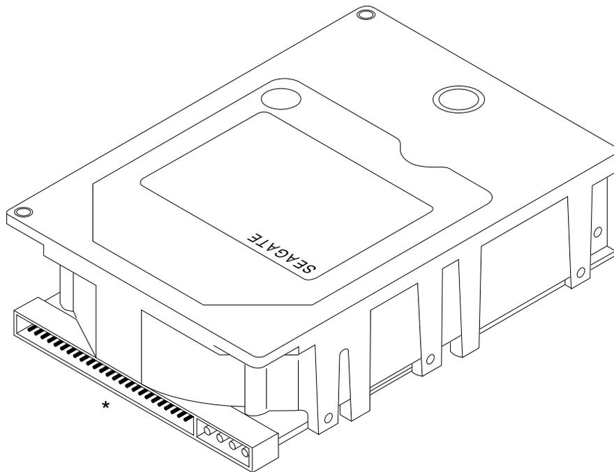
\* 50 pin SCSI I/O and 4 pin DC power connector shown. "NC" drive models have a single 80 pin connector and no separate DC power connector.
