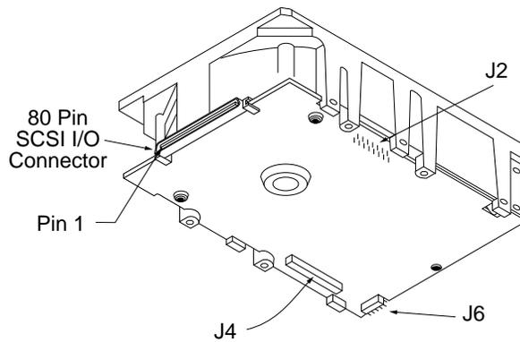
Figure 11.6-1b. "NC" model drive physical interface (80 pin I/O and DC power connector)
