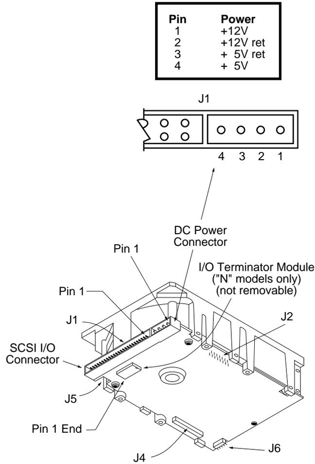
Figure 11.6-1a. "N" and "ND" model drives physical interface (50 pin SCSI I/O connector)
